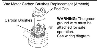
**Note:** When replacing carbon vac motor brushes loosen wire terminal **BEFORE** removing screws on bracket.
